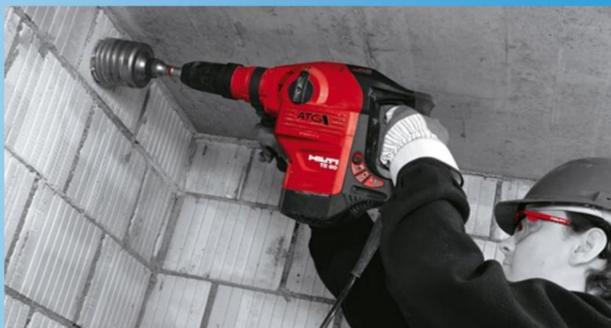
For wet coring: Water suppressed to eliminate dust
